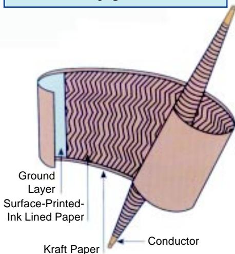
Figure 1 - Surface-printed-ink condenser.
