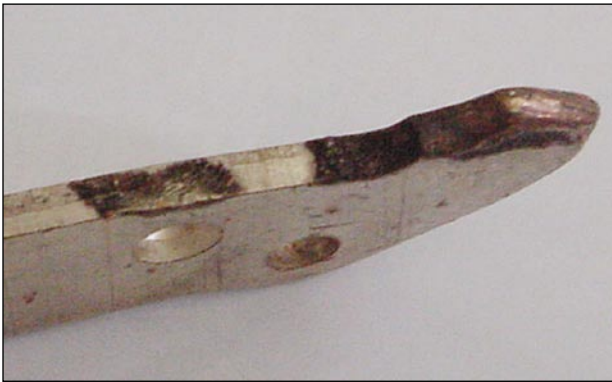
Figure 10b — C-Phase Contact After a Short Circuit
