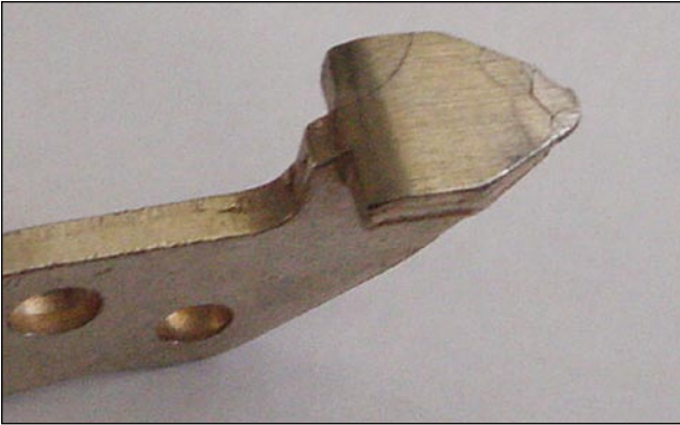
Figure 10a — A-Phase Arcing Contact Showing Cracks in Face
